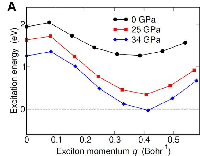
Indirect band gap semiconductor showing at high pressure condensation of excitons at finite momentum.
